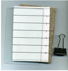
The exposure frame is made up of a piece of thin board (hardboard, thin plywood etc), a piece of bubble-wrap or thin foam rubber the same size for equalising pressure, a piece of thick paper or thin card to cover the foam or bubble-wrap and a sheet of glass the same size as the backing board. 4 sprung clips are used to hold these components together.
